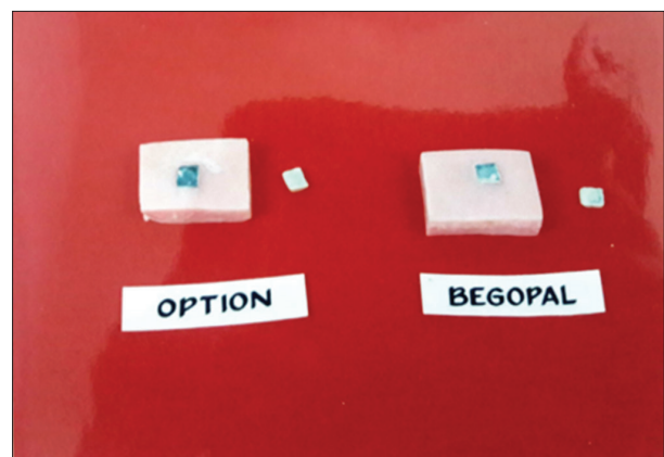
Figure 2: Metal-ceramic specimen of Option and Begopal after debonding
