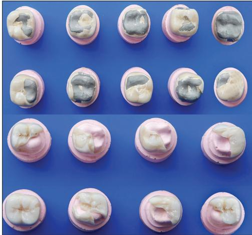
**Figure 3:** Load to fracture tested digital metal laser sintered samples, load to fracture tested zirconia samples
