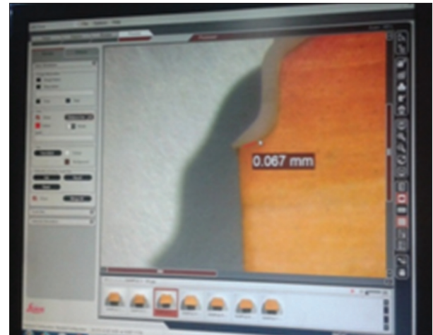
Figure 4: Sectioned crown measured for marginal fit in stereomicroscope
